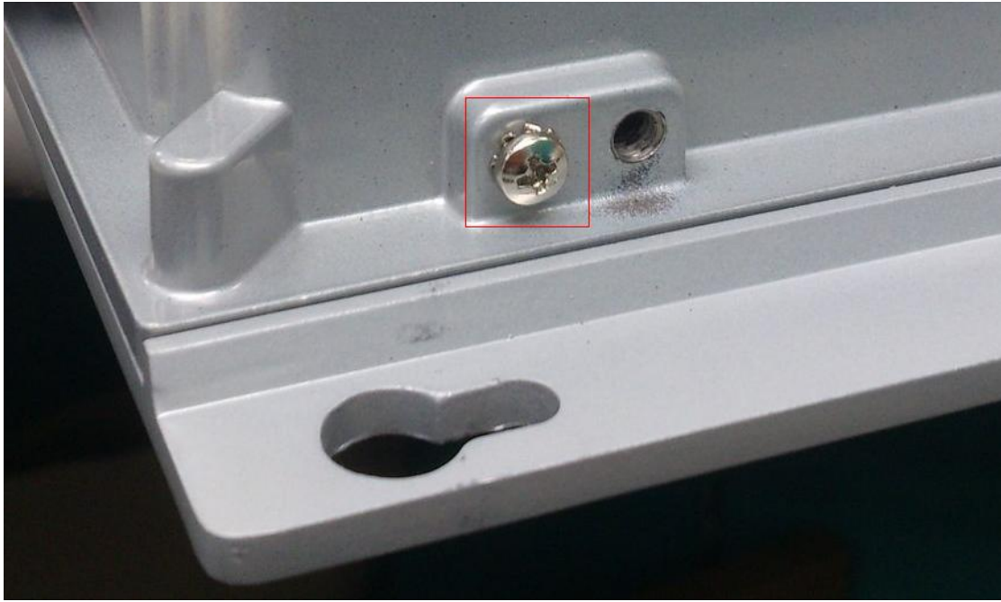
Ground screw of IPES-0008A switch
