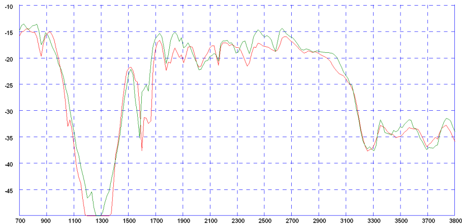
Typical Isolation - Cellular Elements 2&3*
