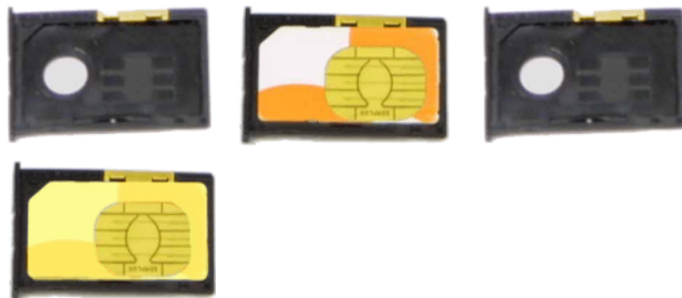
Figure 0-3: Empty SIM Tray and a Tray with a Sample SIM
